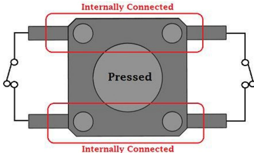
This means that to make it work properly all we need is to connect one pin to a GPIO pin of the Raspberry Pi (I chose pin 32, a.k.a. GPIO12) and the other to GND. We can leave untouched the other two pins of the button.
