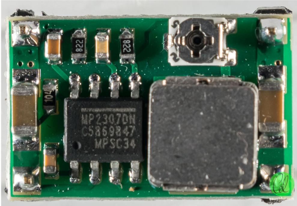
P+ of the BMS gets connected to the positive input of the DC-DC buck converter, while P- will be connected to an on-off toggle switch. One of the output of the toggle switch is connected to the negative input of the buck converter in order to close the circuit when the toggle is on. Finally the positive output of the buck converter is connected to a 5V pin of the Raspberry Pi 3, while the negative output is connected to a GND pin.
