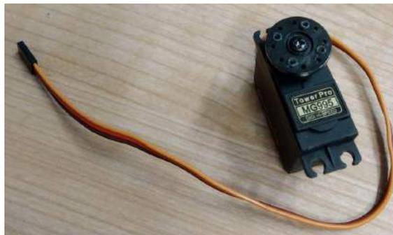
Figure 4: Servo RC 13 kg\*cm
